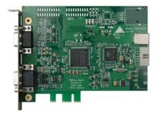
The Sync Board hardware option enables RS-422, LTC, MIDI and optional Bi-Phase to control or to be controlled by VCube.
